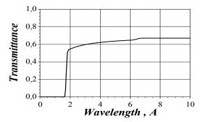
**Figure 8.** The calculated spectral transmission through one channel of analyzer with the mask at its entrance for spin-up neutrons.
