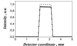
**Figure 7.** The calculated spatial distribution of spin-up neutron intensity passing through the analyzer with a mask at its entrance. The solid line corresponds to neutron intensity for  $\lambda$ =2Å, the dash line for  $\lambda$ =3Å.
