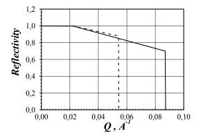
**Figure 2.** Reflection coefficients for the spinup neutrons for supermirrors with  $m_1 = 4$  at the FS wall (solid line) and  $m_2 = 2.5$  at the BS wall (dash line) as functions of Q.
