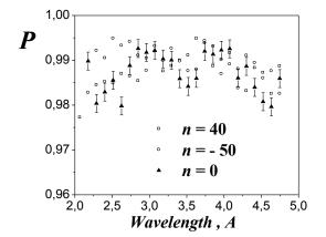
**Figure 9.** Spectral polarizing efficiency for three analyzer channels (n = 40, 0, -50).
