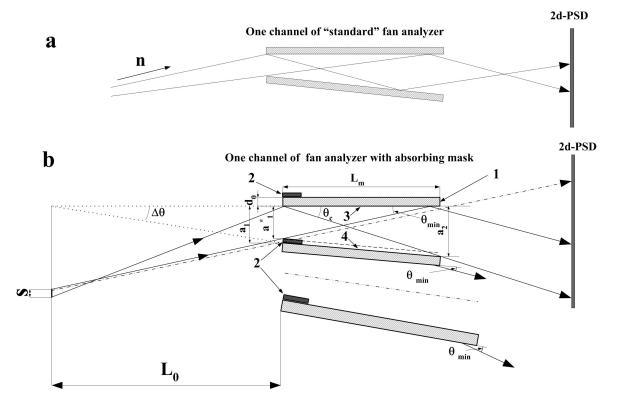
**Figure 6.** Layout of a conventional analyzer (a) and the analyzer with the neutron absorbing mask at the entrance (b). 1 - glass substrate with thickness  $d_0$ ; 2 - absorbing mask; 3 - FS wall; 4 - BS wall.
